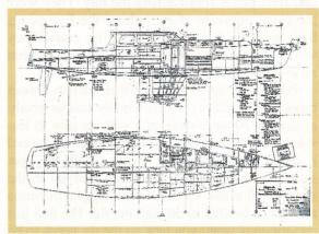
masts keep overall rig weight down. The SA/D is a healthy 29.9, but it has to be high with this rig because there are no jibs or chutes to augment the rig when it gets light. We'll just have to wait and see if this is the ultimate offshore rig. I prefer stayed rigs for offshore work.
