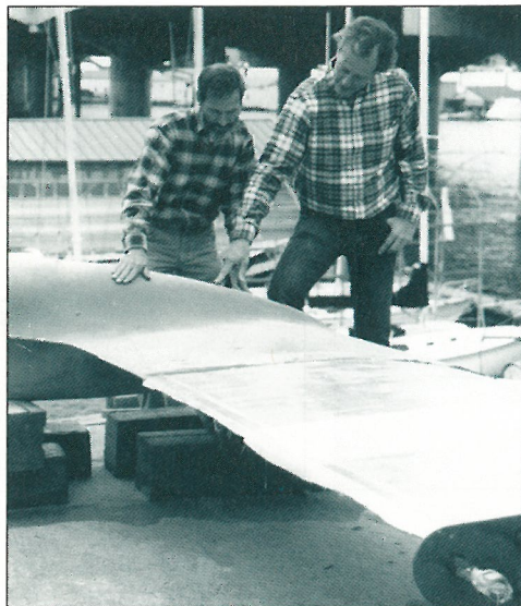
Schooner Creek's Steve Rander ( at left ) and designer Tom Wylie examine the bulb keel before the fin is fastened to the boat ( far left ). Inside the hull, keel loads are distributed to the centerline box girder through a galvanized-steel keelbolt box ( below ).
