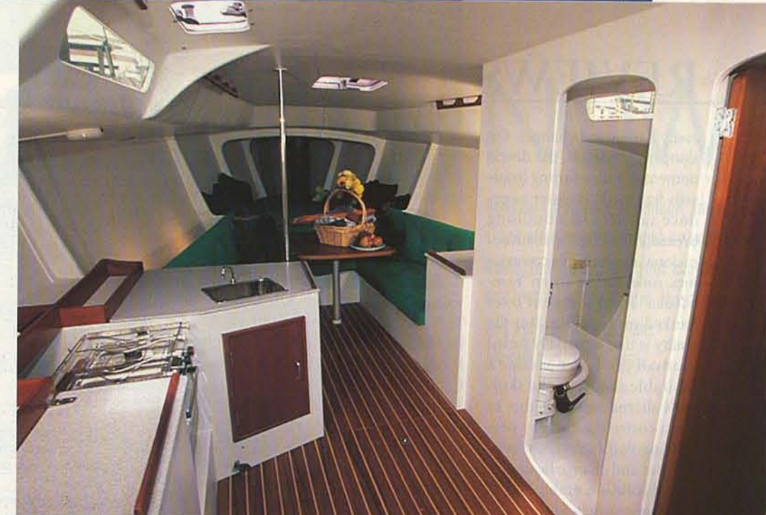
One of the catboat's biggest advantages is hidden below the deck. No rigging means much-reduced rigging loads. And that means the hull structure doesn't rely heavily on bulkheads, so any number of interior designs are available. Ahava's owner preferred a simple, open plan.
